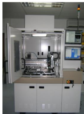
Research Specialist Arlene Orr visually inspecting the tips on the Rainmaker3 before a piezo dispense print to produce a high density NAPPA. Photo by Andy DeLisle
